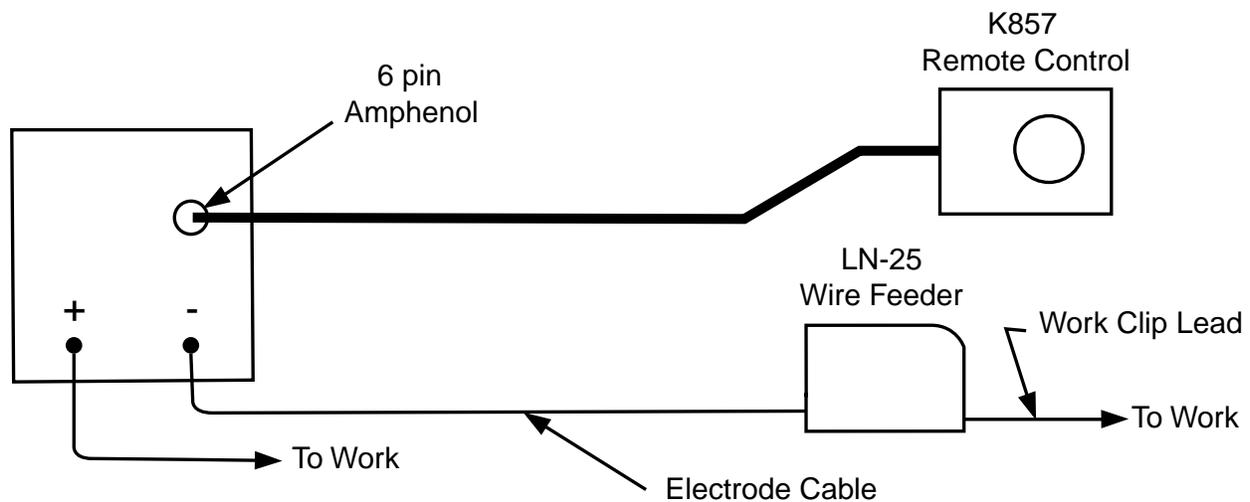
**NOTE:** Illustration shows electrode connected for negative polarity.
