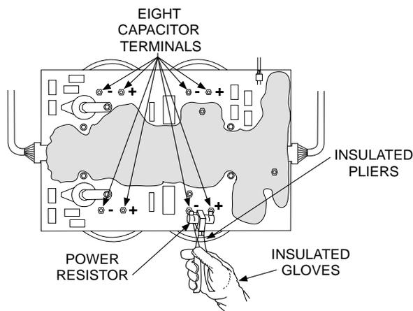
5. Locate the eight capacitor terminals shown in figure D.1.
