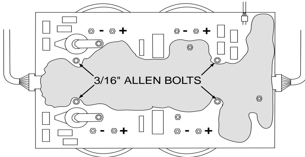
9. Using a 3/16" allen wrench remove four allen bolts and washers as shown in Figure F.24. At this point, the board is ready for removal. Carefully remove the board from the 4 nylon mounting pins. Note: Depress the retaining pins on the sides of the nylon mounts to release the board. See Figure F.25.
