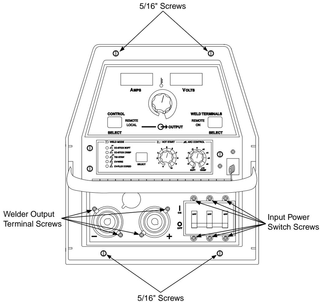
5. Using a 5/16" nut driver remove the four screws from the top and bottom of the front of the machine. See Figure F.22.
