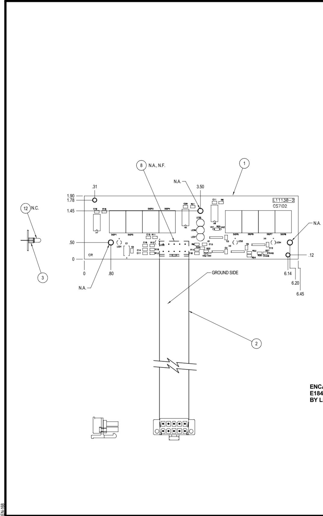
ENCAPSULATE WITH HUMISEAL 1A27LU PER E1844 OR WITH EQUIVALENT AS APPROVED BY LINCOLN ELECTRIC COMPANY. (2 COATS)
