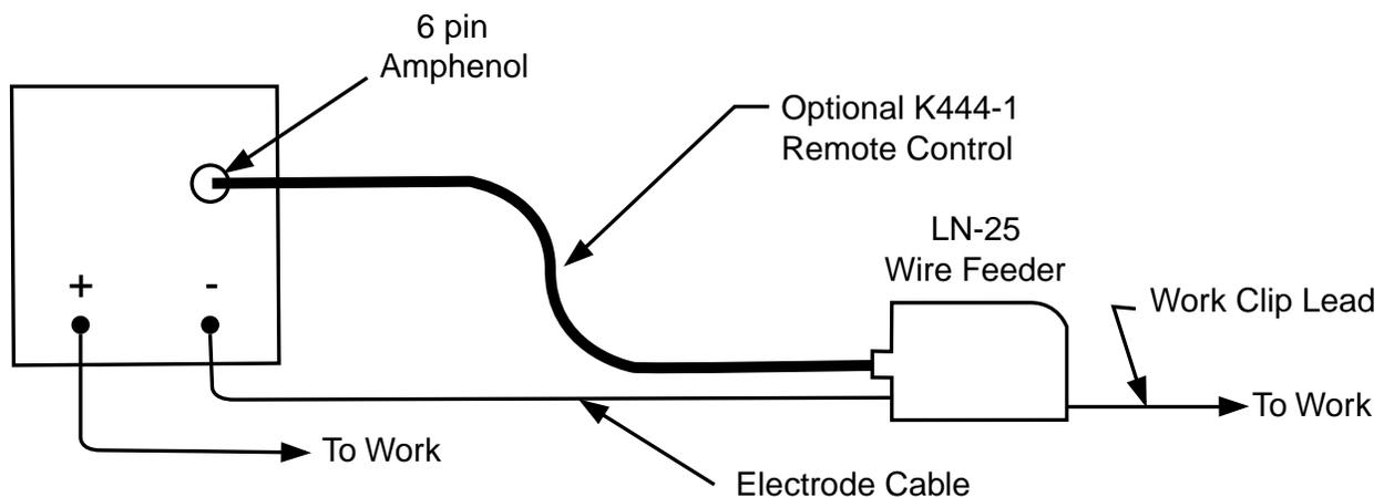
**NOTE:** Illustration shows electrode connected for negative polarity.
