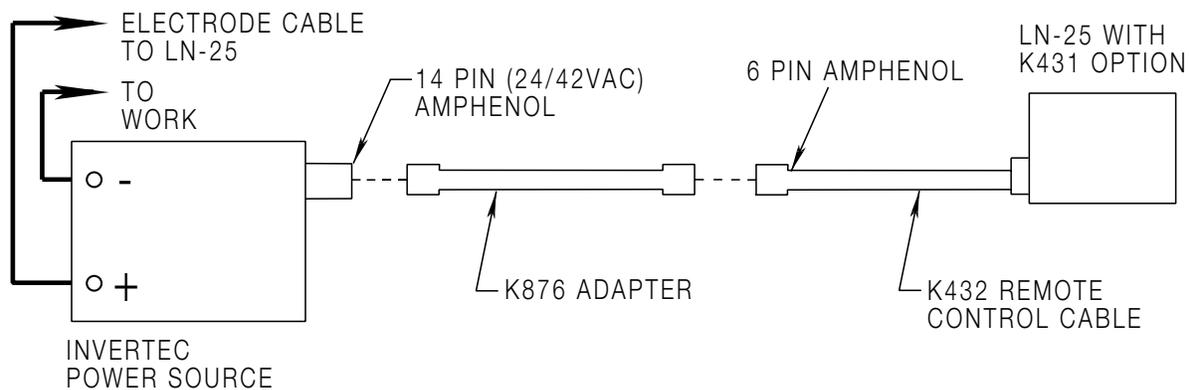
**NOTE:** Illustration shows electrode connected for positive polarity.
